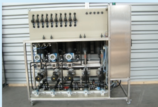
Peripheral devices such as pumps, pressure sensors and flowmeters.
